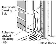
Figure 36 - Installing Thermostat Sensing Bulb behind Glass Doors
